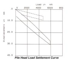
The parameters of most value are generally the distribution of soil resistance down the pile shaft and beneath the pile toe, and the computed pile head load settlement curve. This analysis is generally conducted in the office subsequent to the field testing but can easily be performed on site if rapid answers to anomalous behaviour are required, or to optimise driven pile lengths.
